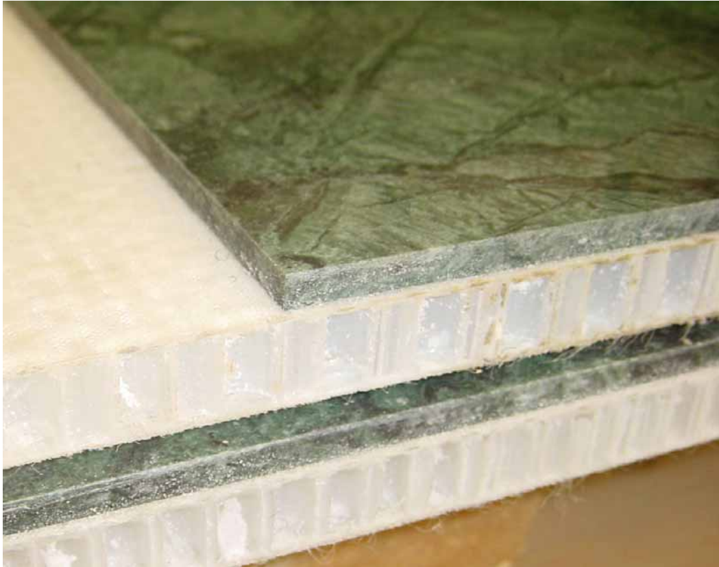
Incollaggio del marmo al pannello Honeycomb Coupling between the marble slabs and the honeycomb panels
